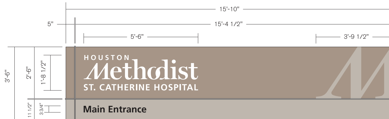
4 13.04 - Large Wall Sign (Subcopy) - Front Elevation (55.4 Sq. Ft.) Scale: 3/8" = 1' - 0"
