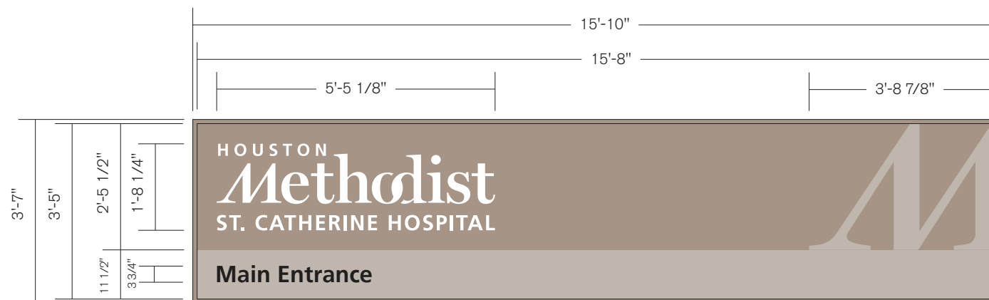
4 14.04 - Large Re-facing Panel - Front Elevation (56.7 Sq. Ft.) Scale: 3/8" = 1' - 0"
