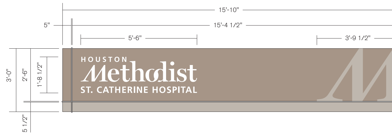
4 13.02 - Large Wall Sign - Front Elevation (47.5 Sq. Ft.) Scale: 3/8" = 1' - 0"
