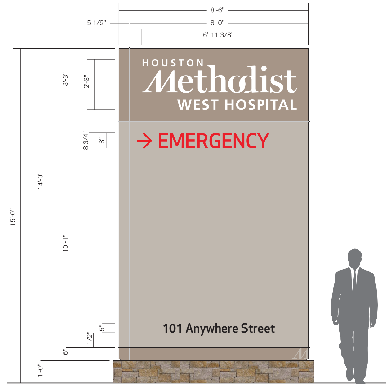
2 4.01 - Large Site Identifier - Front Elevation (142.5 Sq. Ft.) Scale: 3/8" = 1' - 0"
