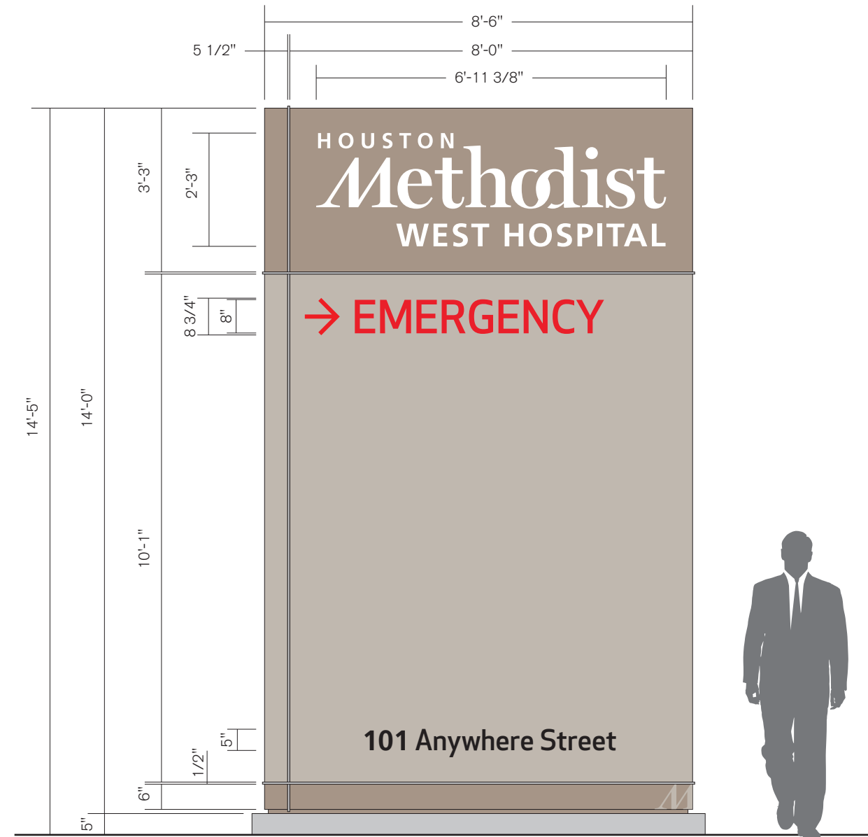
2 5.01 - Large Site Identifier - Front Elevation (122.5 Sq. Ft.) Scale: 3/8" = 1' - 0"
