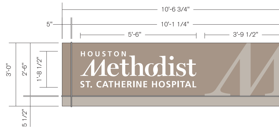
2 13.01 - Small Wall Sign - Front Elevation (31.75 Sq. Ft.) Scale: 3/8" = 1' - 0"
